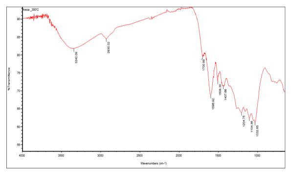
Figure 6 FTIR spectra of Areca nut Husk Biochar
