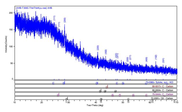
Figure 4 XRD analysis of Areca nut Husk Biochar
