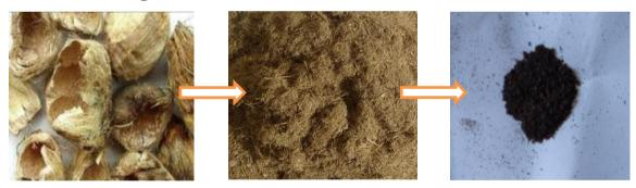
Figure 2 Conversion of Areca nut Husk biomass into Biochar
