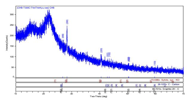
Figure 3 XRD analysis of Coconut Husk Biochar
