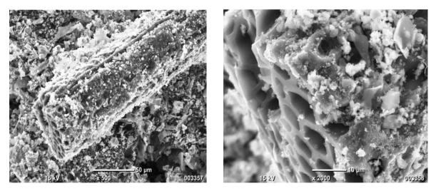
Figure 8 SEM image of Areca Husk Biochar at (a) 500 X and (b) 2000X magnification
