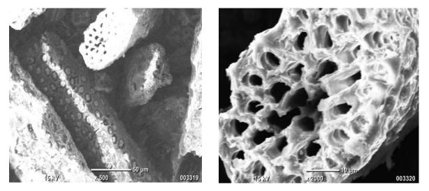
Figure 7 SEM image of Coconut Husk Biochar at (a) 500X and (b) 2000X magnification
